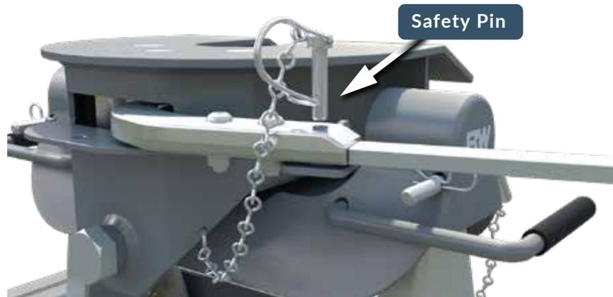
4. Use the safety pin to lock the handle in the open position and when you are sure that the landing gear will support the trailer, move the truck forward to release the jaws from the kingpin.
